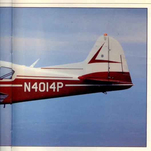
in Wichita according to a supplemental type certificate obtained by Doyne Conversions (now defunct). The modifications consisted of the replacement of the Apache's 160-hp engines with 180-hp Lycoming O-360-A1As and the addition of both a dorsal fin and another window in the fuselage.
